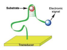
How apt these sensors are! Electronic aptamer-based sensors (aptasensors) hold great promise as analytical devices for the detection of low-molecular-weight substrates or proteins. The Minireview highlights the advantages of electronic transduction of aptasensor systems and discusses the latest developments in the design of electrochemical, field-effect transistor, and piezoelectric aptasensor systems.
